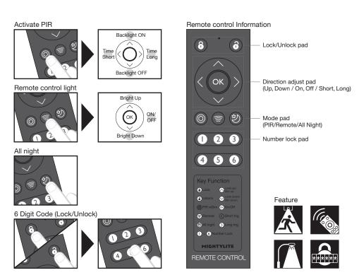
If you forget your 6 digit code, disconnect the battery on the floodlight and reconnect again. This will delete the code on your remote control.
