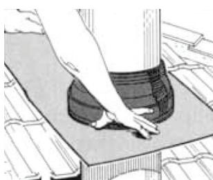
Slide the tile roof flashing down over the tube to the tile roof level. Water can be used as a lubricant.
