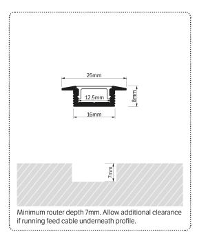
XR2508 Premium extrusion comes complete with plastic end caps and an opal frosted diffuser.
