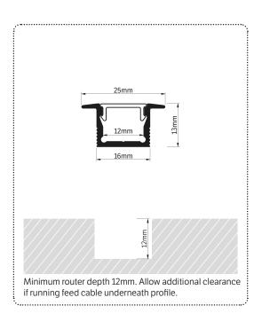
Premium extrusion comes complete with Aluminium end caps and opal frosted diffuser.
