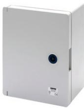
Range of Watertight surface-mounting boards made in thermoplastic material GW PLAST 120. In compliance with IEC 61439-1 (CEI 17/113), IEC 61439-2 (CEI 17/114), IEC 60670-1 (CEI 23/48) e IEC 60670-24 (CEI 23/49). Available in 4 sizes, transparent and black door versions with IP55 protection degree. Accessories available: panels with window complete with extrable frames, for modular devices and moulded-case circuit breakers up to 160A. Indicated for automation and distribution.
